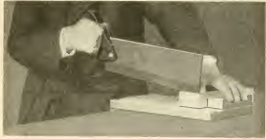
Fig. 4. Sawing Cross Grain on Bench Hook with Back or Handy Saw.
